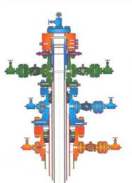
typical conventional wellhead consists of a lowermost casing head housing with casing hanger, an intermediate casing head spool with casing hanger and tubing suspension equipment including tubing head spool and tubing hanger.
